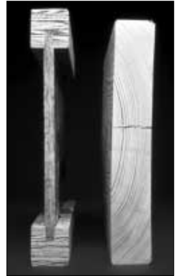
I-Joists use 50% less wood fiber than solid sawn lumber.
