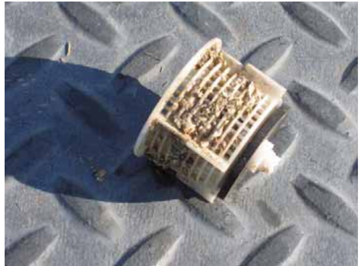
FIGURE 2 SNAIL INFESTATION IN ROHNERT PARK RECYCLED WATER DISTRIBUTION SYSTEM
