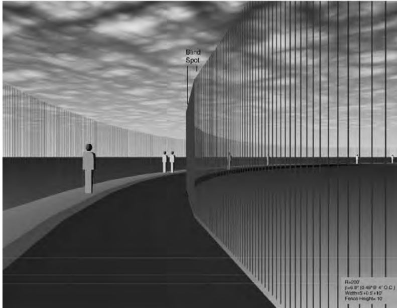
Figure 3.6 Blind Spots on curved pathways.
